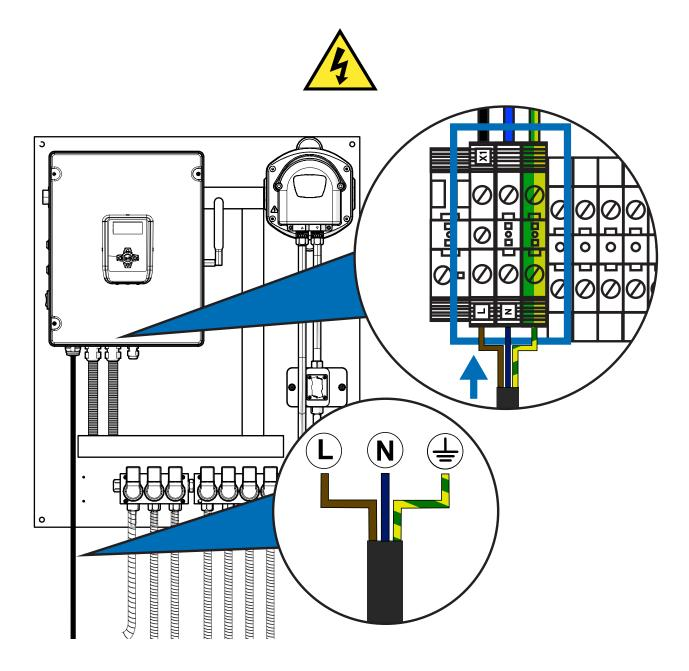
For the power supply of the equipment you must use **3x1'5mm2 cable**. Insert the cable through the channel located at the bottom left and use one of the cable glands to insert it safely inside the control cabinet. Connect to the terminals identified with **X1** found on the lower left of the connections.
