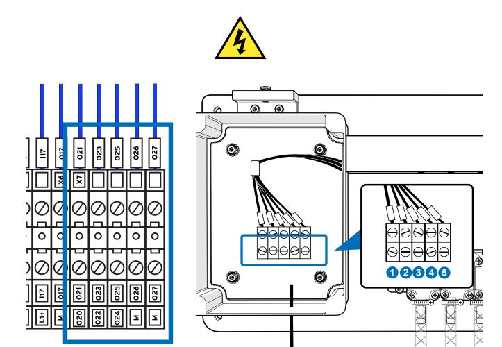
Use a 7x1mm^2 cable for the connection between the control cabinet and the distributor. Connect the distributor to terminal block X7. Each terminal connection corresponds to the outlets numbered from left to right, with the number dependent on the order. Below is the wiring diagram for the main unit.
