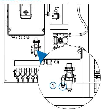
There are 3 connectors located on the underside of the control panel related to air on the Multiplex 2 Pro. You only need to connect the one labelled 1.
